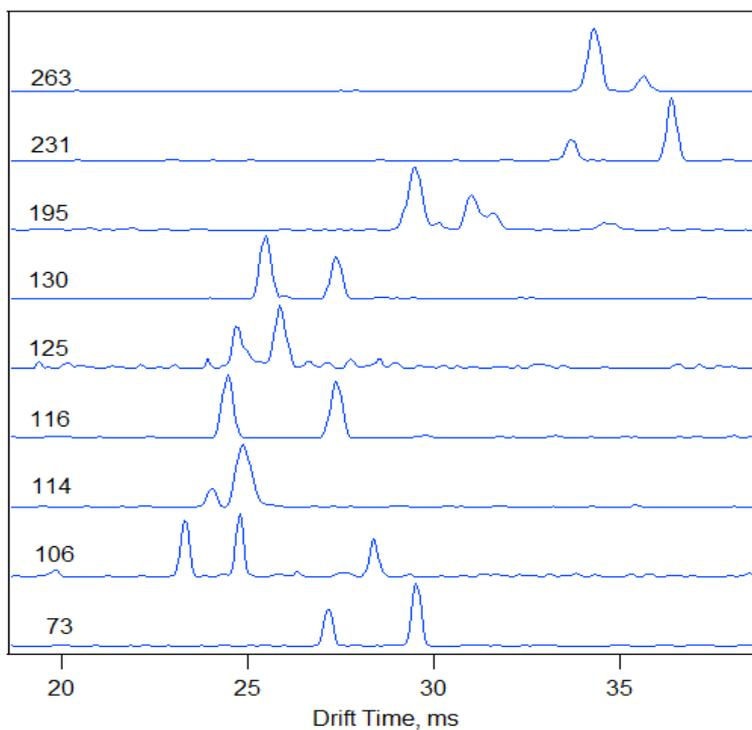
Whisky headspace IMS traces. The nominal masses are indicated. Each peak in each trace represents an isomer or isobar which was not resolvable in the mass spectrum.
