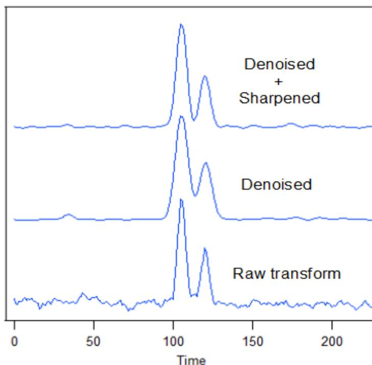
Example of combined denoise and sharpening. Denoise broadens, sharpening reduces S/N. Together, the final result is both resolved and has high S/N.
