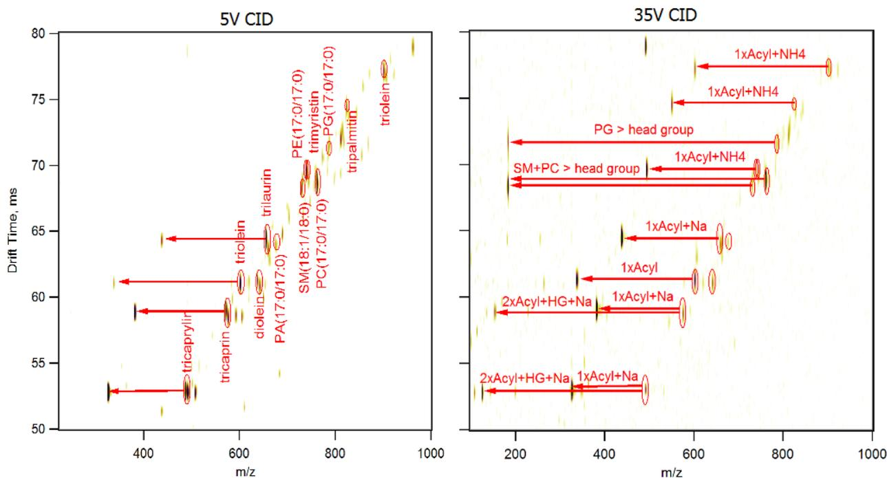
Lipid mixture IMS-TOF diagram at low post-drift collision energy (left) and high collision energy (right). Relatively few fragments are observed at 5V, while characteristic side chain and headgroup fragments are abundant at 35 V. Due to drift time separation, assignments are easy and unique.
