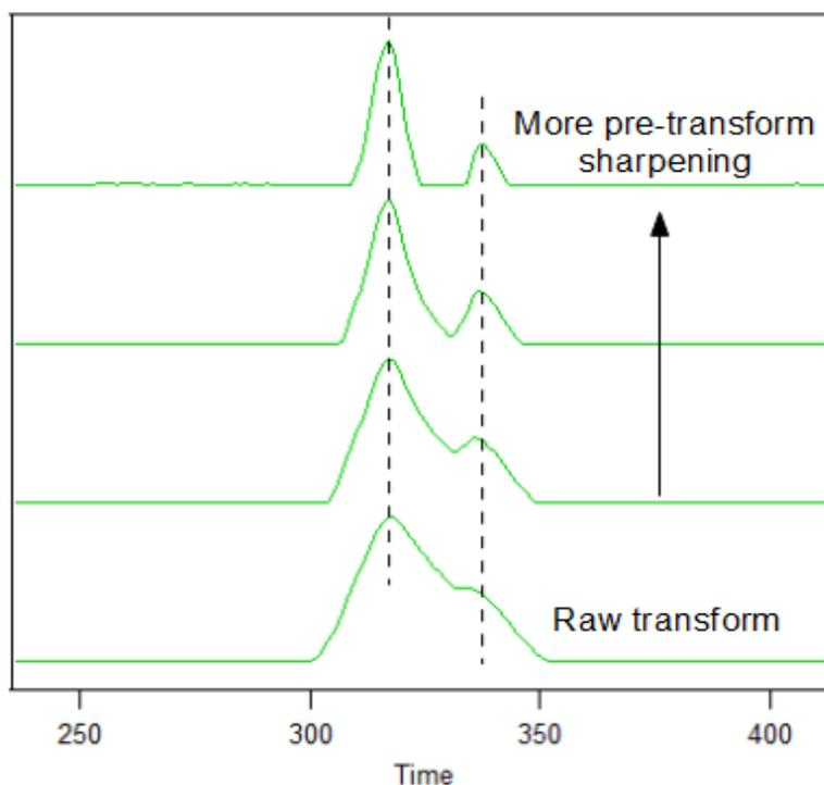
Example of the effect of sharpening in the multiplexed domain. Peak positions and relative intensities are retained.
