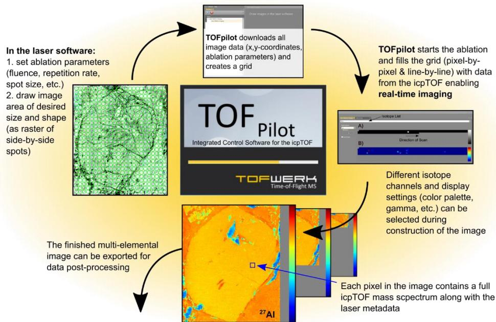
Figure 4 Workflow diagram for the Laser Ablation Imaging Module in TOFpilot. In this example, a 6 mm by 7 mm garnet crystal was imaged. The multi-element image was recorded at a laser repetition rate of 100 Hz, spot size of 20  $\mu\text{m}$ , fluence of 3 J/cm<sup>2</sup>, and Dosage 1 (laser shots per pixel). Here only the <sup>27</sup>Al image is shown. The entire range of elements was recorded simultaneously in ~55 min.
