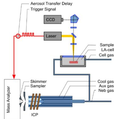
Figure 2 Schematic of precise triggering. Based on synchronized communication between the laser ablation system and the icpTOF (via a TTL cable) a trigger pulse is sent with every laser shot to start the data acquisition at the icpTOF. The delay time between ablation and detection (aerosol transfer delay) depends on the sample material and on the conditions within the ablation cell and must be calibrated prior to analysis.
