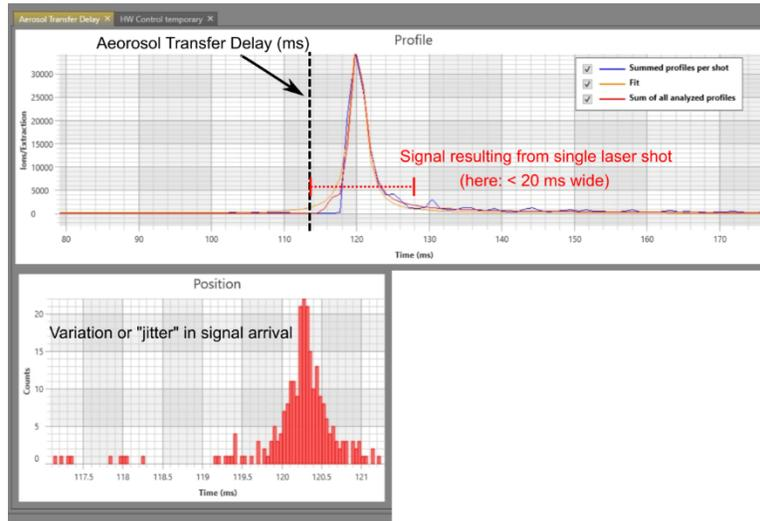
Figure 3 Aerosol Transfer Delay Module in TOFpilot. The signal from a single laser pulse is shown (<20 ms). The delay can be shifted so that it is within the integration window accounting for pulse-to-pulse jitter.
