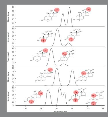
Separation of isomeric progesterone metabolites commonly found in urine. Using the TOFWERK IMS-TOF and electrospray ionization, laborious sample preparation as commonly done for GC analysis is avoided. The high ion mobility resolution allow confident detection and quantification of isomers that cannot be separated by LC. The instrument was operated with the following settings: IMS pressure 1000 mbar, IMS temperature 70°C, nitrogen as drift gas.
