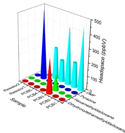
**Figure 1** Four selected substances emitted by PCBs and resistors taken from disposed electronics. Dimethylformamide is listed as the dominating specie from PCB samples. The PCB piece which was coated with silicone layer can be clearly differentiated.
