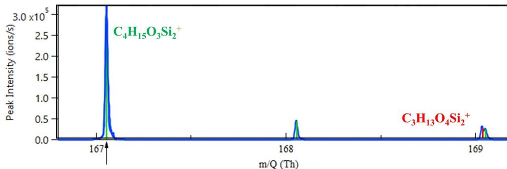
**Figure 2.** Headspace mass spectra acquired from sample 3. The peak identification as Dihydroxytetramethyldisiloxane was both confirmed by exact mass and characteristic  $^{29}\text{Si}$  and  $^{30}\text{Si}$  isotopic pattern (illustrated as green sticks). Due to the high resolving power of Vocus PTR-TOF, another organic silicon compound was clearly identified at the  $m/Q$  169.
