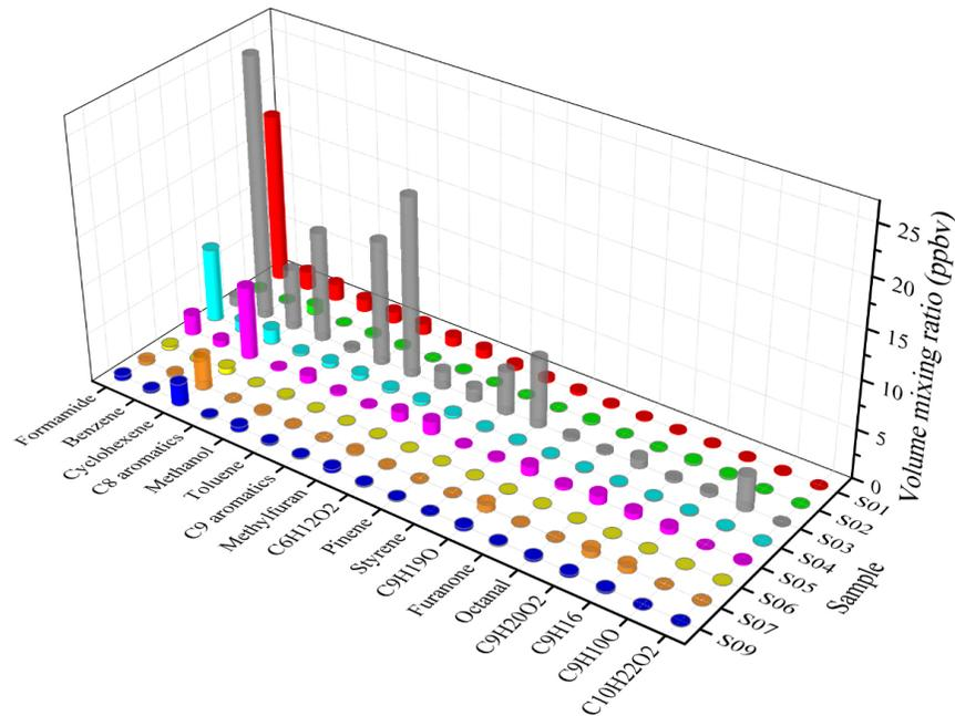
**Figure 3** Additional chemicals observed from the emissions of 8 packing material samples. Sample S03 shows high emissions in aromatics and derivatives, whereas sample S02, S06, S07 and S09 emissions are much lower. Relatively high formamide, which could be from residual process solvent, were obtained in both sample S01 and S04.
