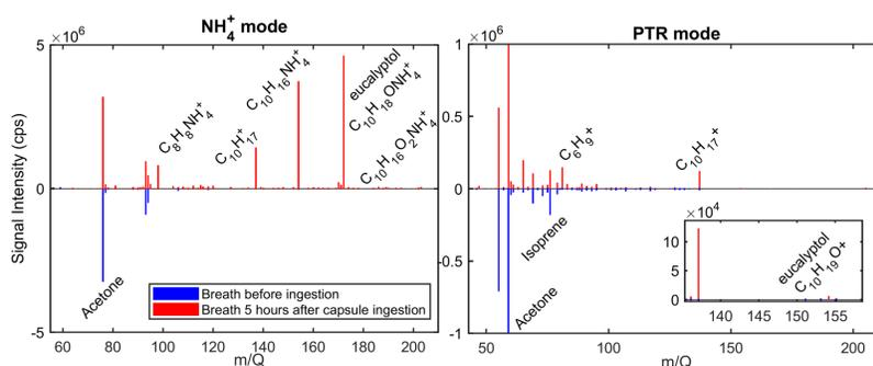
**Figure 2** Mass spectra recorded in  $\text{NH}_4^+$  and PTR mode for one individual before and after eucalyptol oil ingestion.
