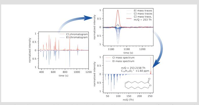
Example application: Parallel recorded CI (red) and EI (blue) chromatograms of a perfume sample resulting in synchronous acquisition of molecular and fragment ion information for improved compound identification via high resolution, accurate mass GC-MS.
