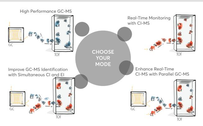
The combination of ion sources and sampling methods yields multiple modes of operation. Different modes generate molecular information by CI and structural information by EI.
