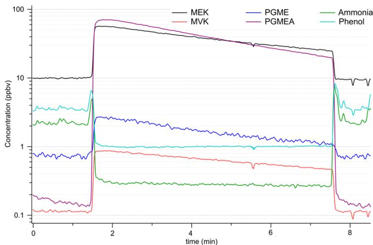
**Figure 6.** Off-gassing of material in an ISO 5 microtechnology cleanroom. Material was purged with CDA and measured directly. Each time series shows simultaneous compound measurements with 3 different ionization chemistries for comprehensive AMC coverage.
