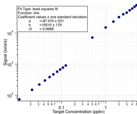
**Figure 3.** Linear range of coverage for toluene.
