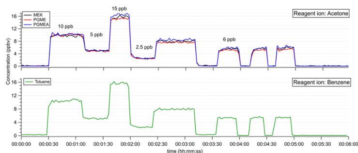
**Figure 1.** Response and recovery time of a ClearFab AMC Monitor. Labels in the plot show target concentrations while the Y-axis shows the measured concentration of selected compounds. The upper plot shows the concentration of MEK, PGME and PGMEA measured with one chemical ionization chemistry, while the lower plot shows the simultaneous measurement of toluene with another chemical ionization channel chemistry.
