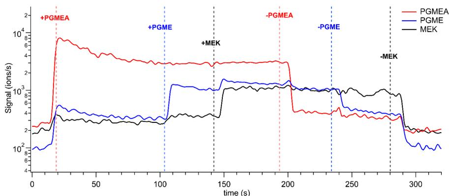
**Figure 2.** Sequential measurement and removal of PGMEA, PGME and MEK demonstrating the detection of these challenging compounds without fragmentation.
