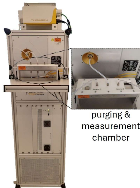
Figure 1: Vocus 2R PTR from TOFWERK used for the detection of solvent emissions (leak rate) from batteries. Leaking battery purged by a VOC-free gas inside the measurement chamber (right).
