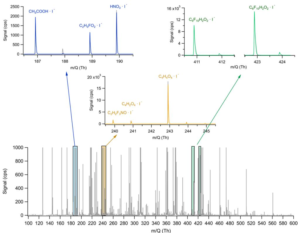
**Figure 3.** Example mass spectrum from a cleanroom ISO 6. Several compounds are monitored simultaneously, independent of their AMC category or mass. Low mass molecules (blue), medium mass molecules (yellow) and high mass molecules (green).
