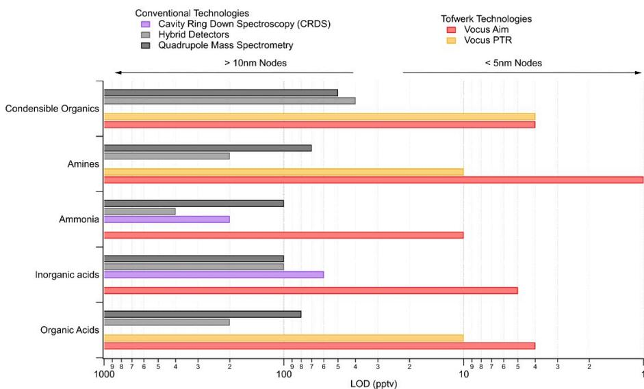
**Figure 2.** Comparison of Vocus CI-TOF and other technologies used for AMC monitoring.
