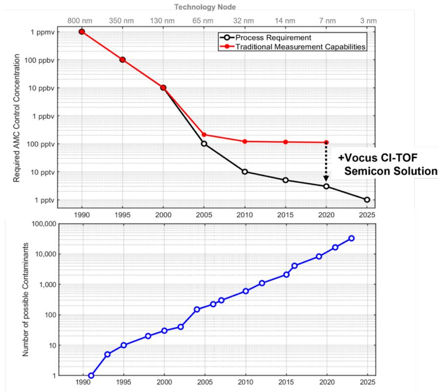
**Figure 1.** Figure 1. Upper - Changes in technology have drastically reduced required AMC control concentrations across time. Capabilities of traditional AMC measurement techniques have not kept pace. The Vocus CI-TOF closes this gap. Lower - The number of AMC contaminants is increasing as the industry reduces feature size.
