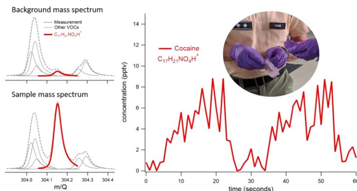
**Figure 1** Vocus TOF analysis of confiscated cocaine. A small bag containing cocaine was opened several times in front of the instrument inlet. Enhancement of the cocaine molecule at ppt levels is observed. The high resolving power of the instrument (Vocus S,  $dm/m=6000$ ) allows the unambiguous measurement and identification of the peak at  $m/Q$  304  $C_{17}H_{21}NO_4H^+$ .
