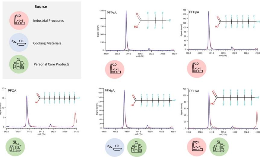
Figure 1. Mass spectra peaks of several PFAS. Red lines: measured spectrum, blue line: calculated isotopic fingerprint for each molecular cluster.
