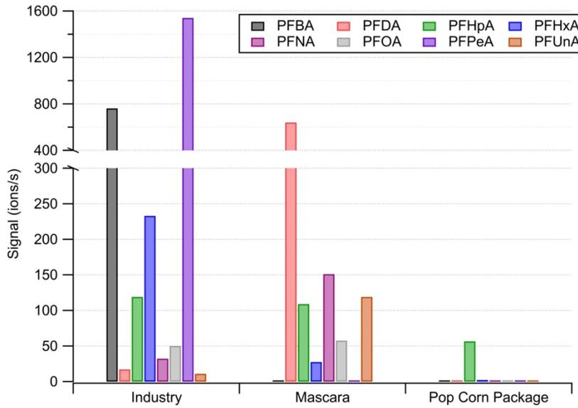
Figure 2. Comparison of PFAS signals in industrial air, waterproof mascara sample headspace, and popcorn sample headspace. Estimated concentrations range from about 5 ppt to 200 pp
