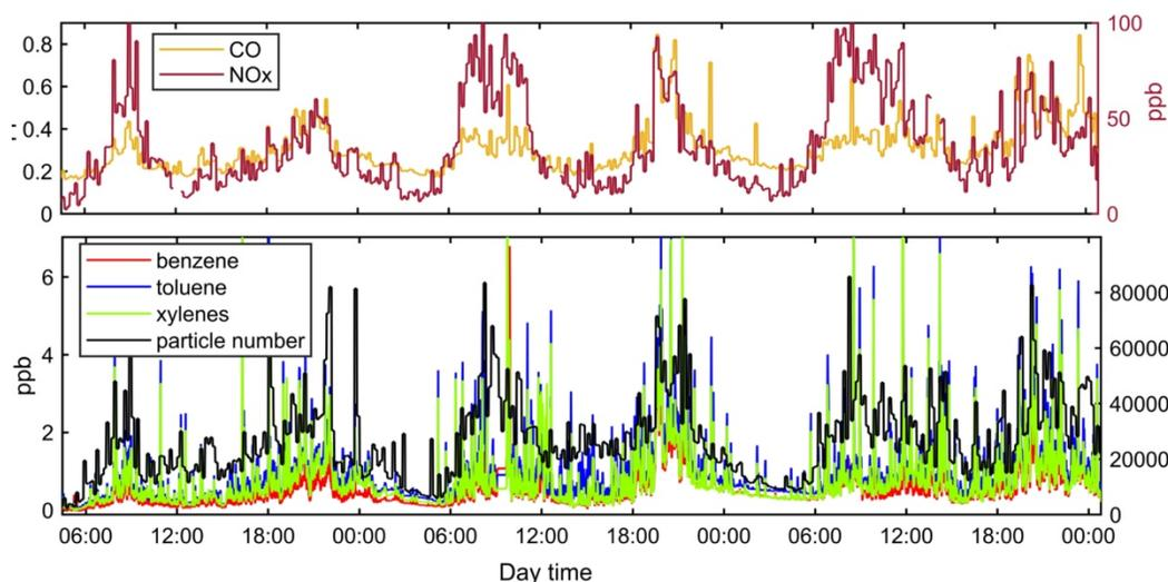
**Figure 3.** (Upper) Measurement of CO and NO<sub>x</sub> during the measurement campaign in Bern Bollwerk. (Bottom) Concentration of BTX measured by Vocus CI-TOF and total particle number measured by CPC.
