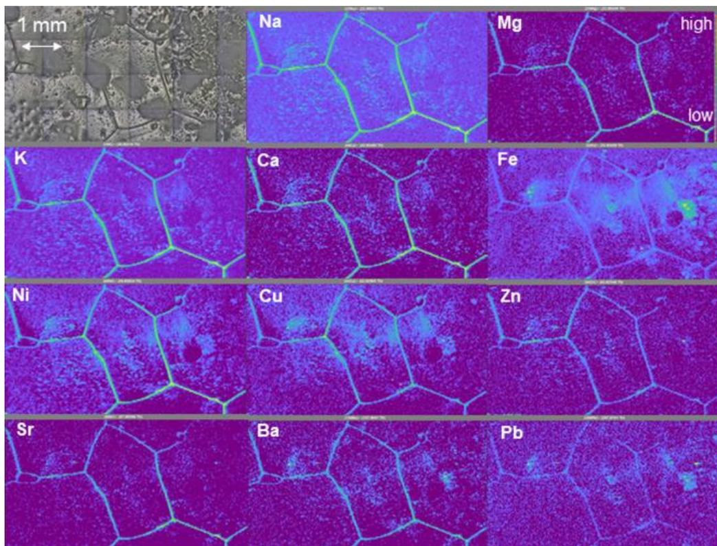
**Figure 1.** LA-ICP-TOFMS images of impurities spatial distribution in Antarctic ice (EPICA Dome C core) from the Holocene time period. The color-scale refers to the raw signal intensity recorded by the icpTOF 2R. Image dimension is 4 mm by 7 mm. The top left corner shows a mosaic of optical images taken with the integrated camera from the same region of interest, where dark lines correspond to the grain boundaries, large dark spots to air bubbles.
