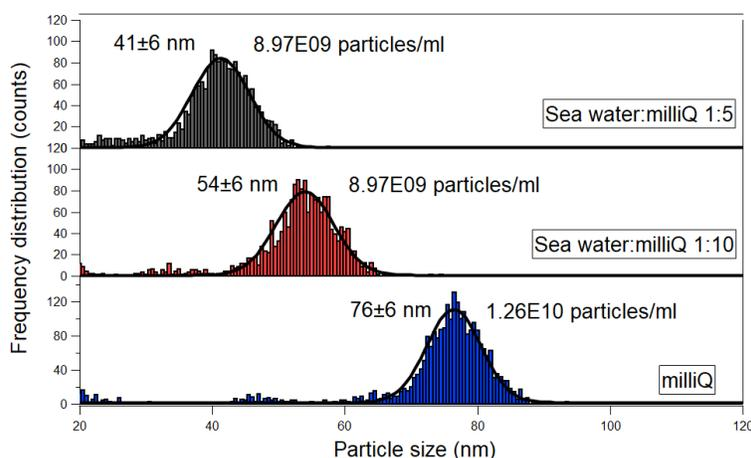
**Figure 1.** Size and particle number concentration of Pt nanoparticles determined using Pace calibration method.
