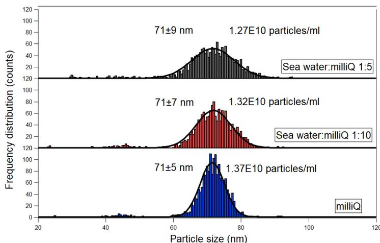
**Figure 2.** Size and particle number concentration of Pt nanoparticles determined by using the combination of the Quantistar and the icpTOF with the online microdroplet calibration method.
